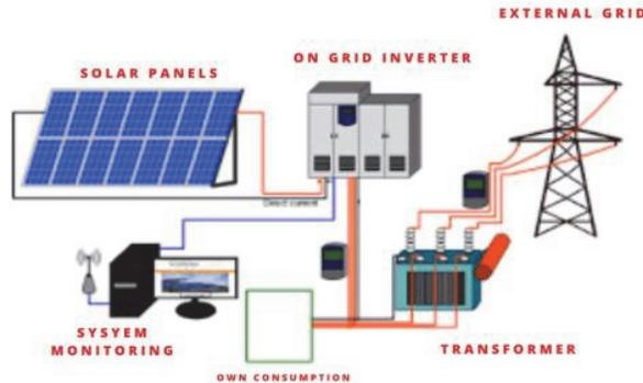
Figure 3. On-grid Solar System Design & Installation
