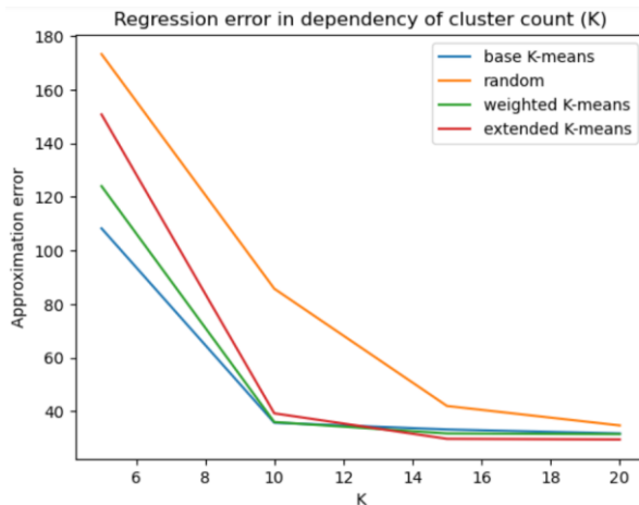
Figure 4. Dependency of the approximation error from the number of clusters (clob data, linear regression-approximation, N=600 , D=5 )
